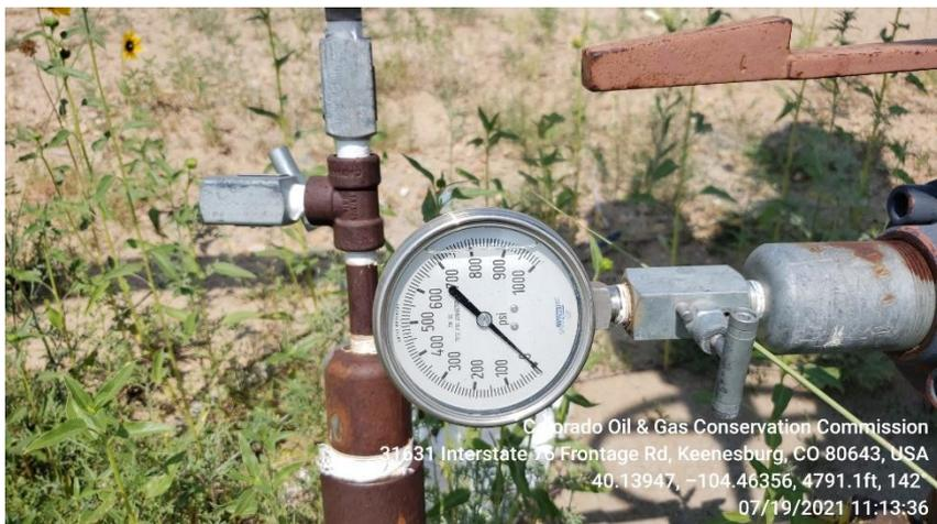
**Photo 5 Casing pressure gauge.**
