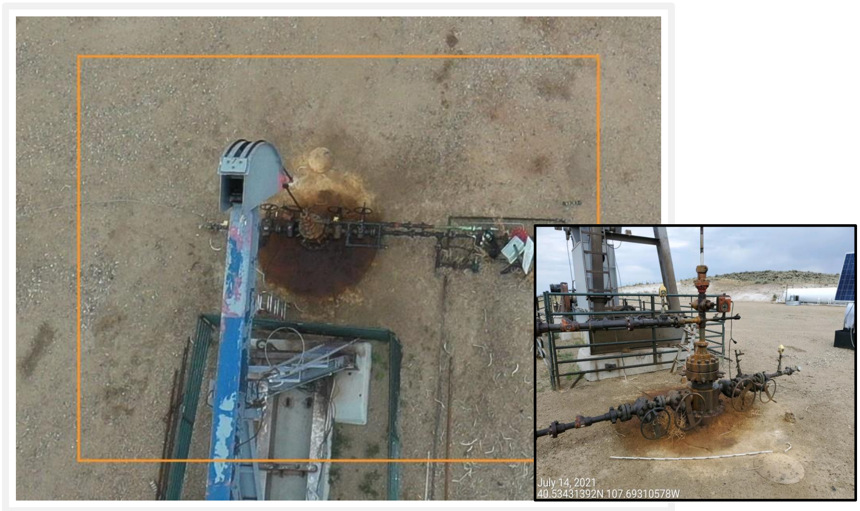
Photo 12: Photo taken from well 081-07817. Photo shows an ongoing release at the well of E&P waste resulting in impacted soils. 6 foot measuring stick for reference.
