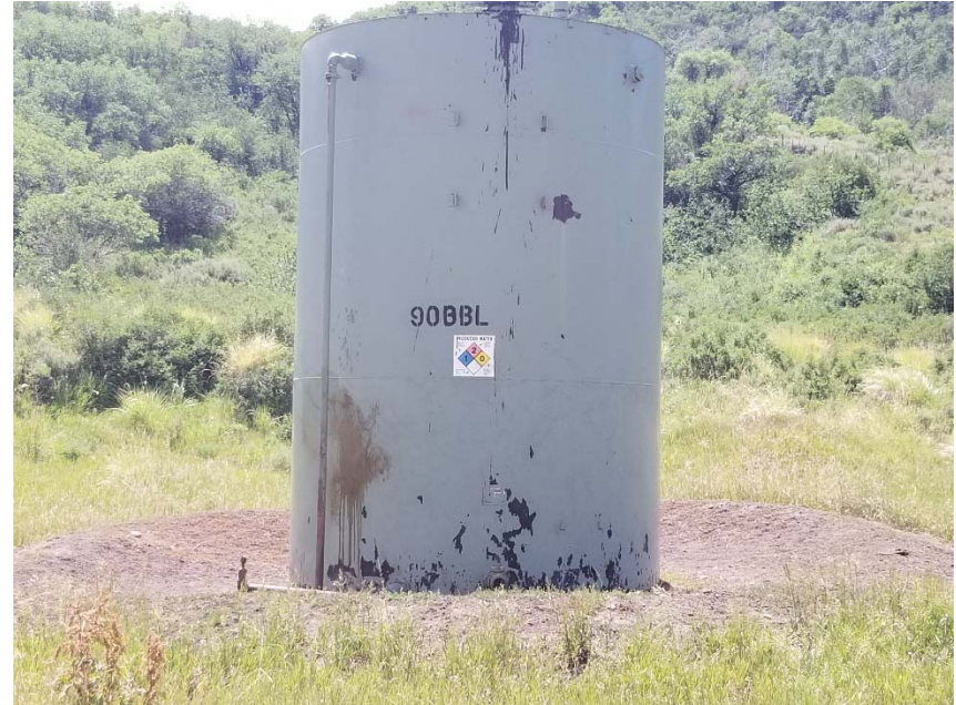
Photo 6. Tank label does not comply with new sign rules.
