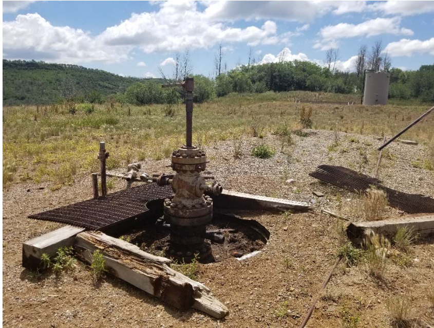
Photo 2. No wellhead sign. No bradenhead access apparent.
