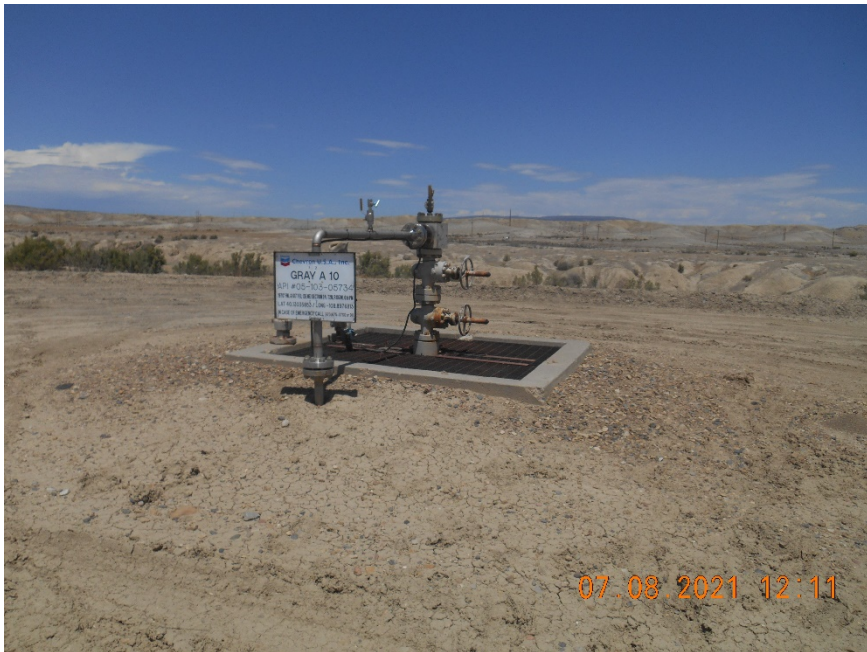
Injection wellhead.
