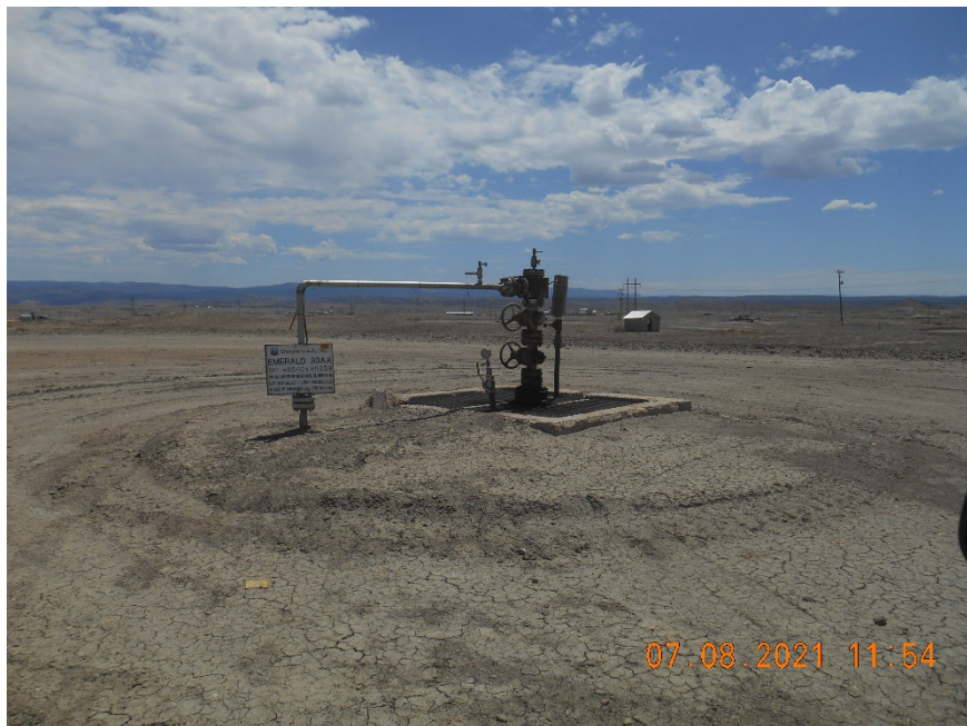
Injection wellhead
