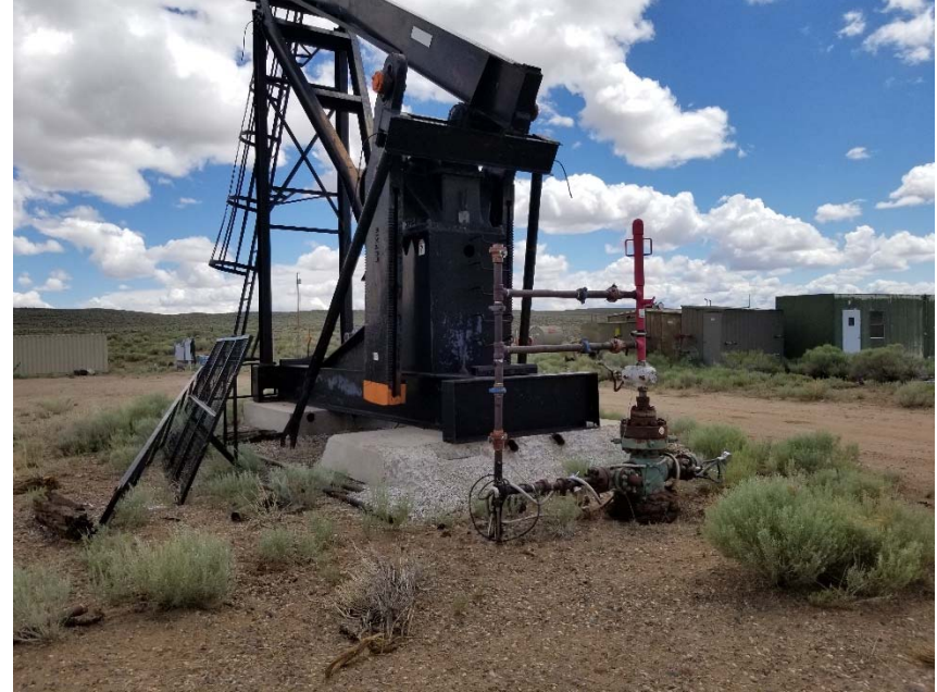
Photo 12. No wellhead sign. No bradenhead access apparent.
