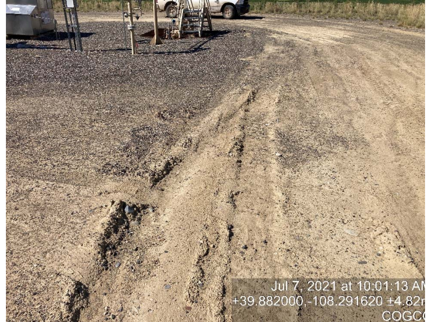
Lack of stabilization/compaction
