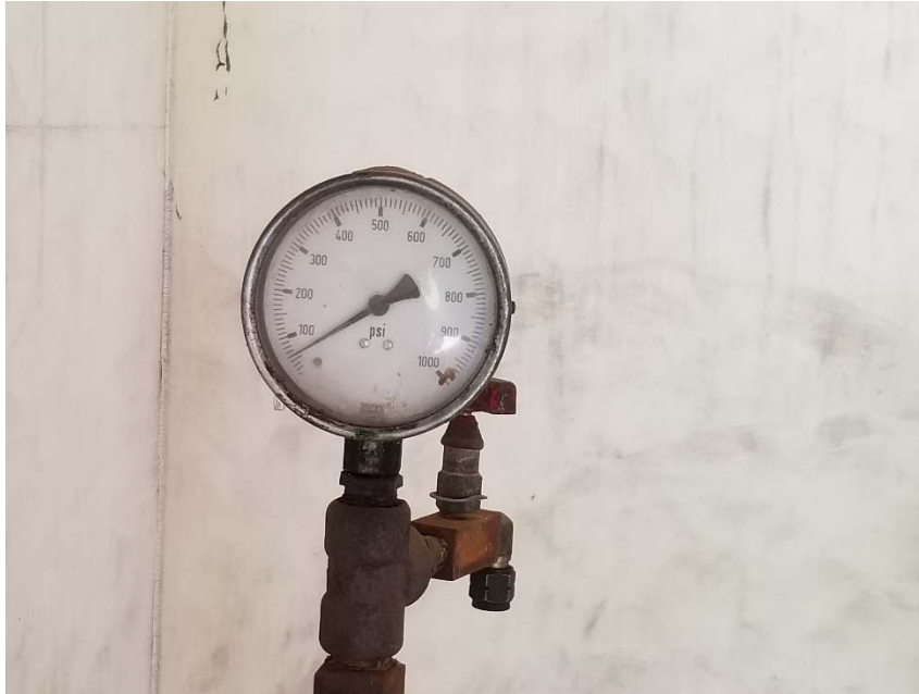
Photo 2. 50 psi on injection tubing at time of inspection.
