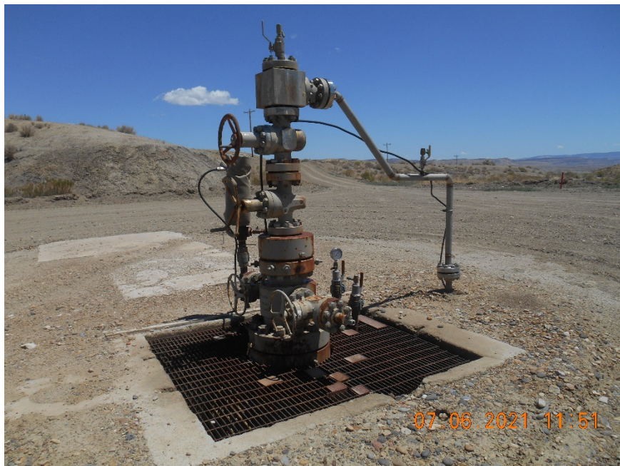
Injection wellhead
