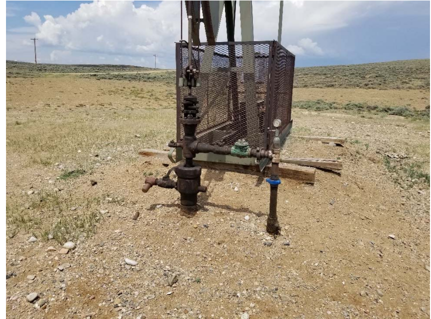
Photo 2. No bradenhead access apparent.
