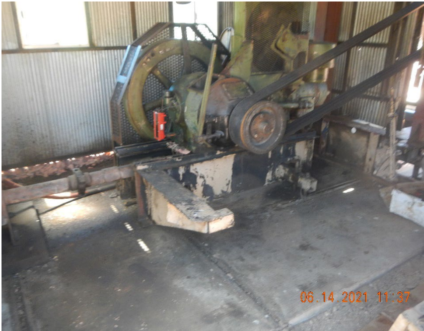
Photo #4 motor drive for Pumpjack.
