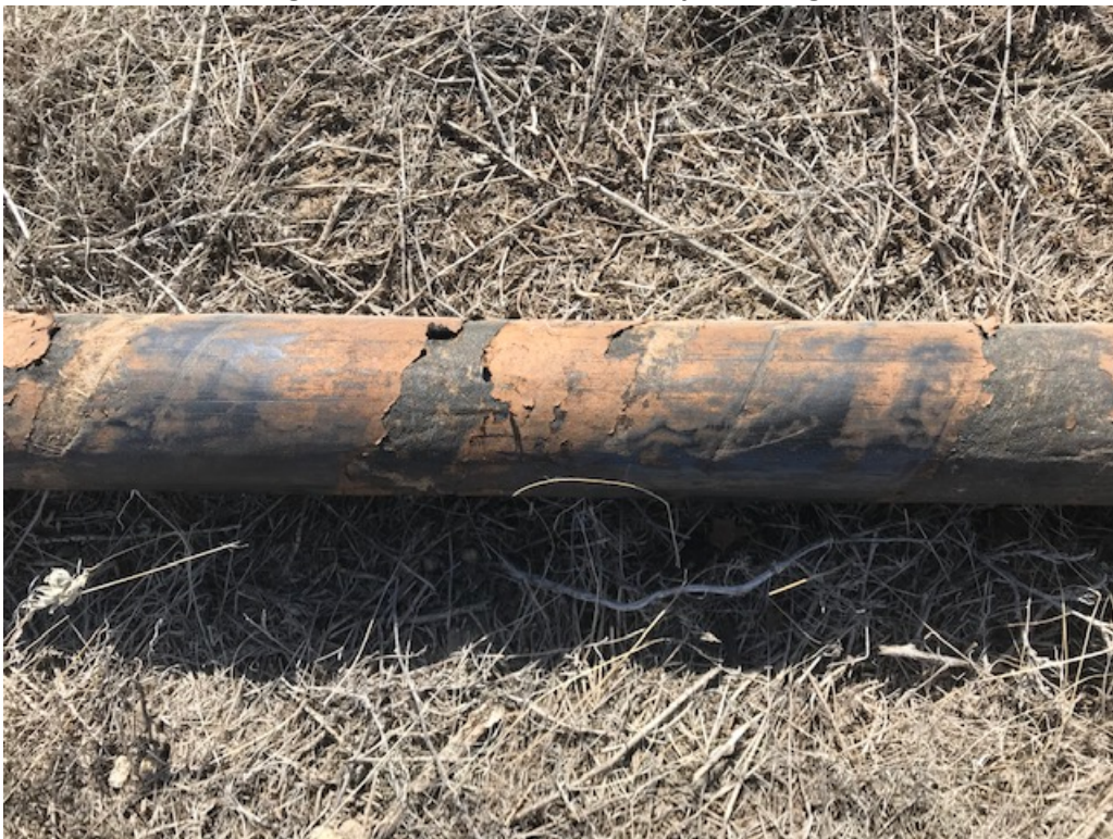
#4 - 2-inch pipe was in good condition. Coating was TGF on ~Sch 40 steel pipe.
