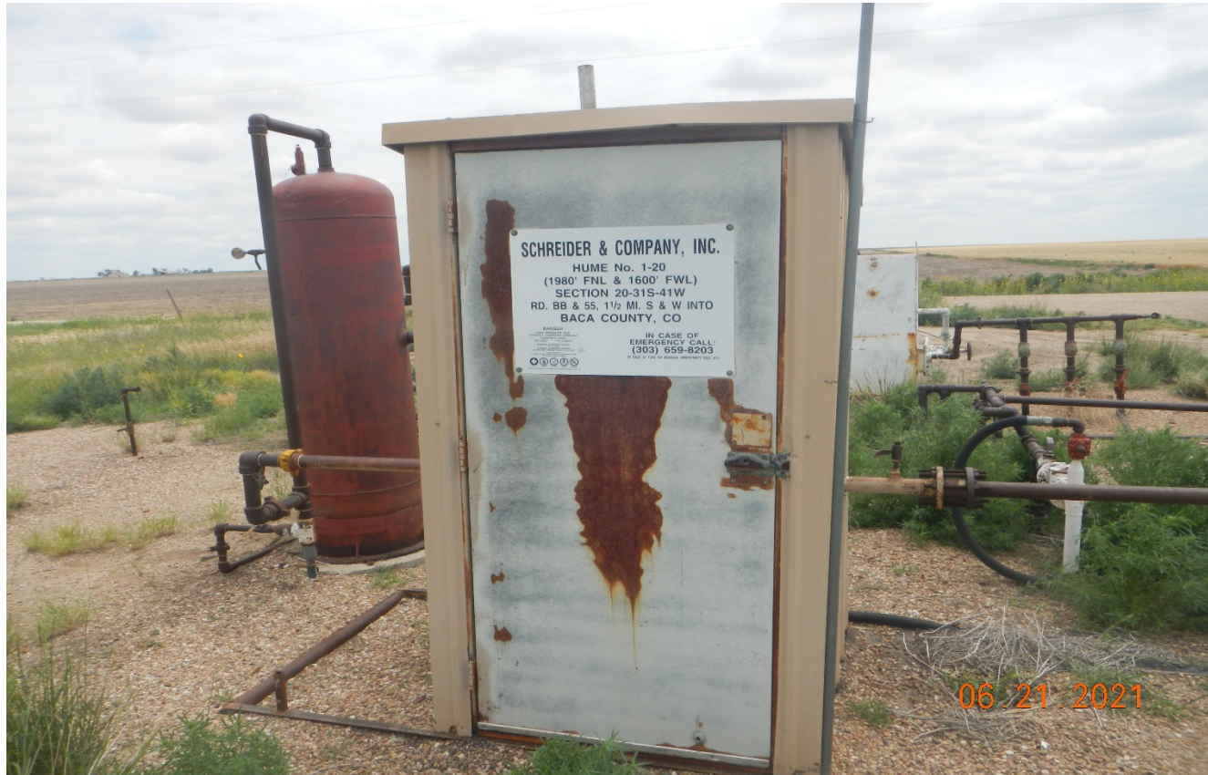
Photo 4. Sign posted at the facility is listed as the Hume 1-20 which the well was plugged and abandoned in 2005. All equipment should've been removed within 3 months of abandonment.
