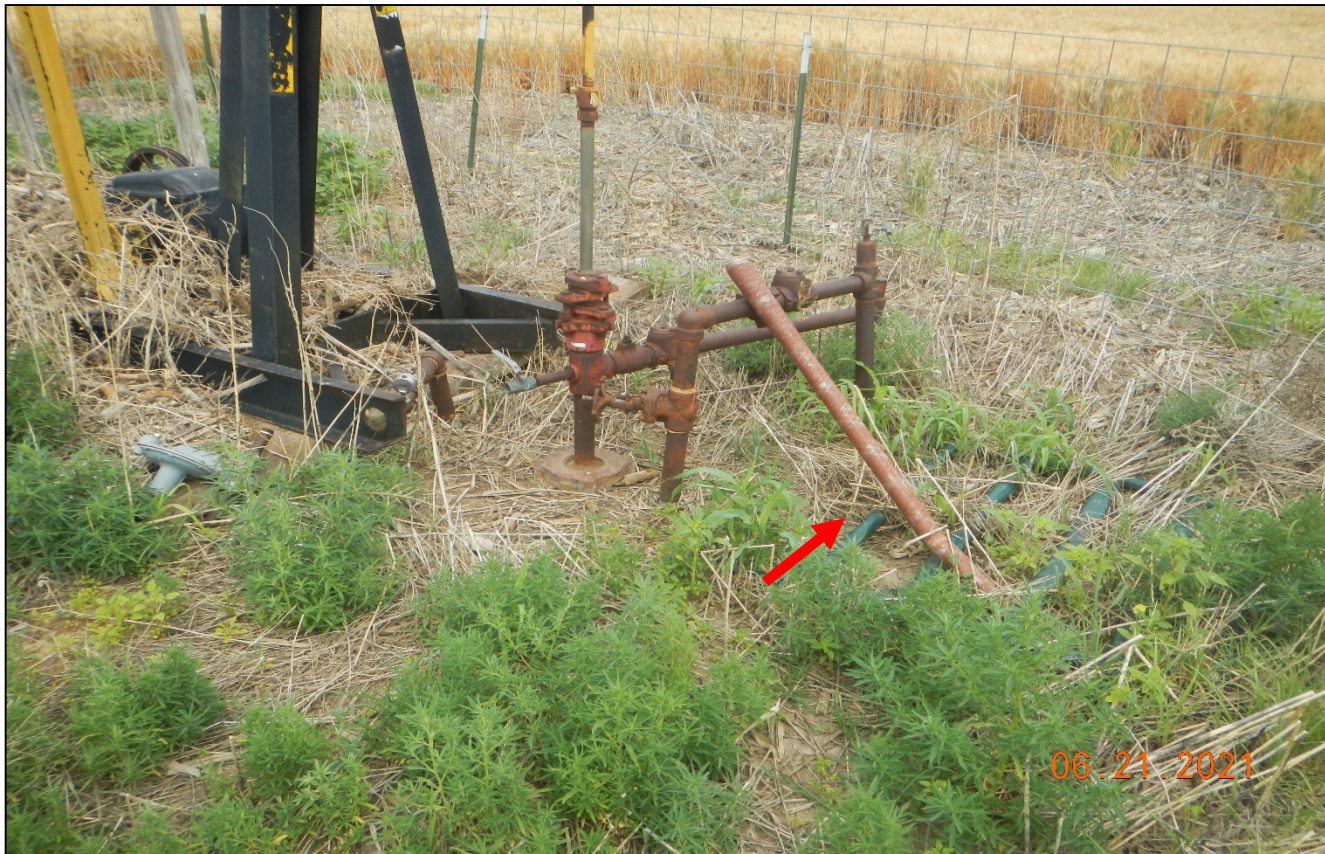
Photo 7. The gate is lying on the ground and the fence around the well is not maintained.
