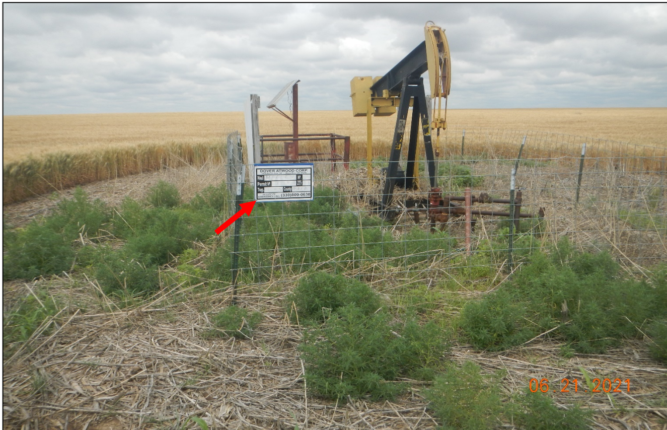
Photo 6. Facing east toward the well. A sign has been posted but is faded and not legible.
