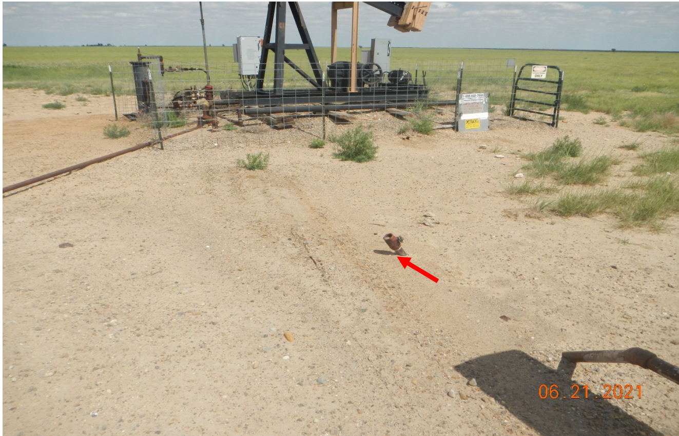
Photo 4. There is a pipe riser shown at red arrow with no LOTO.
