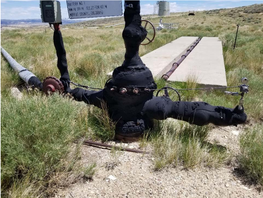
Photo 3. No bradenhead access apparent.
