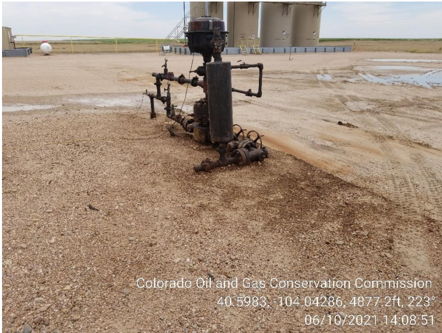
Photo 9 – Stained Soil at Wellhead
