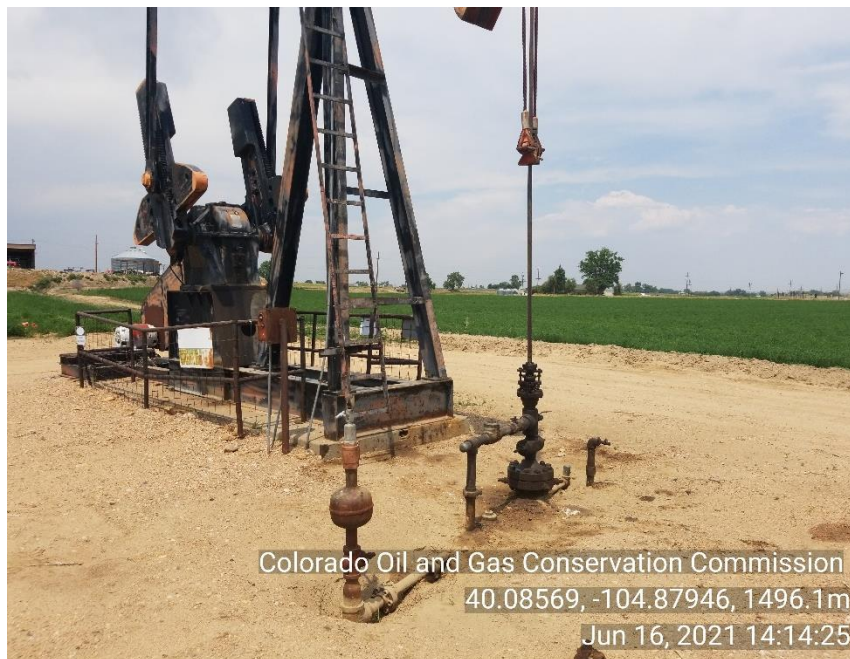
Photo 9 Stained soil around well head.
