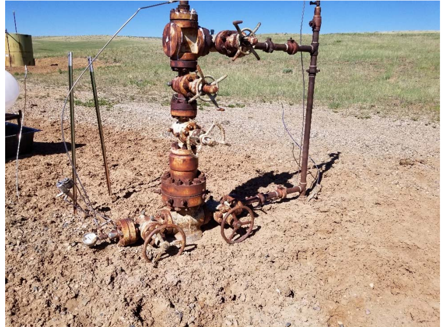
Photo 2. No bradenhead access apparent.
