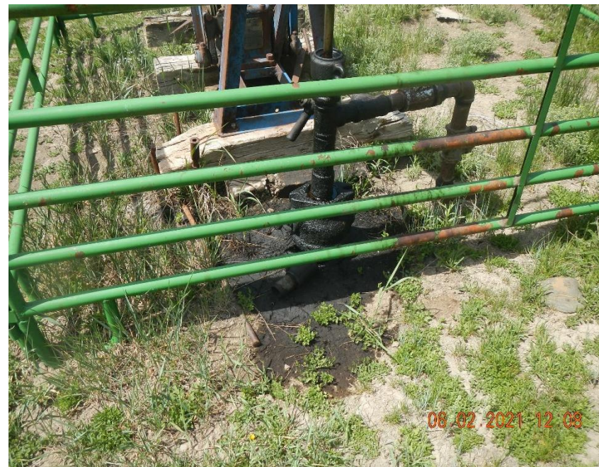
Well head and surrounding area is wet and stained with oil.
