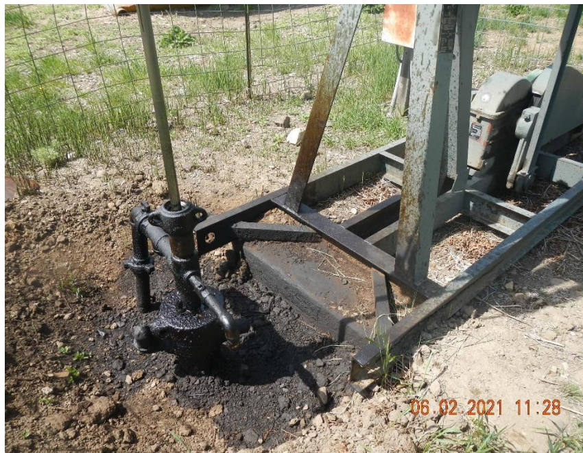
Chavez #1 pump jack and surrounding area is stained with oil.
