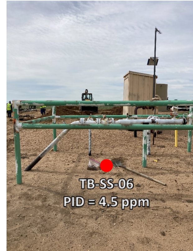
Looking south at above ground gas manifold No petroleum hydrocarbon staining or odor observed
