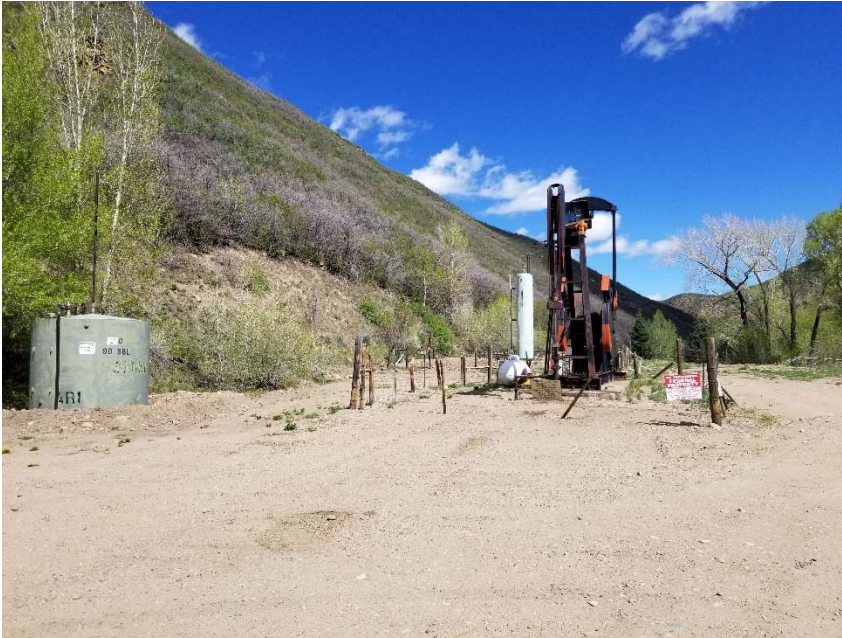
Photo 1. Overview of location taken facing north. Stained soil in front of wellhead.
