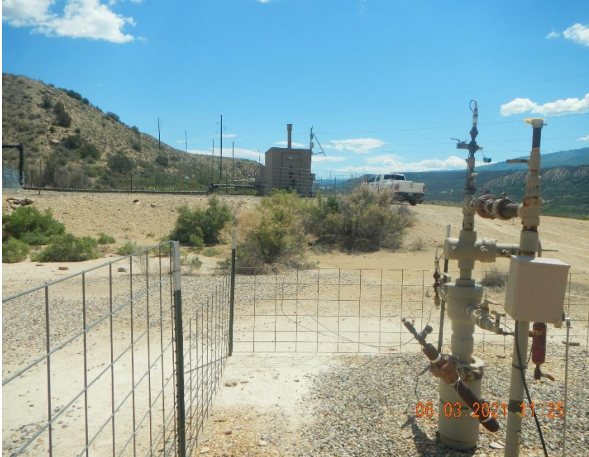
Half inch line from GV W 2-33 to heated separator.
