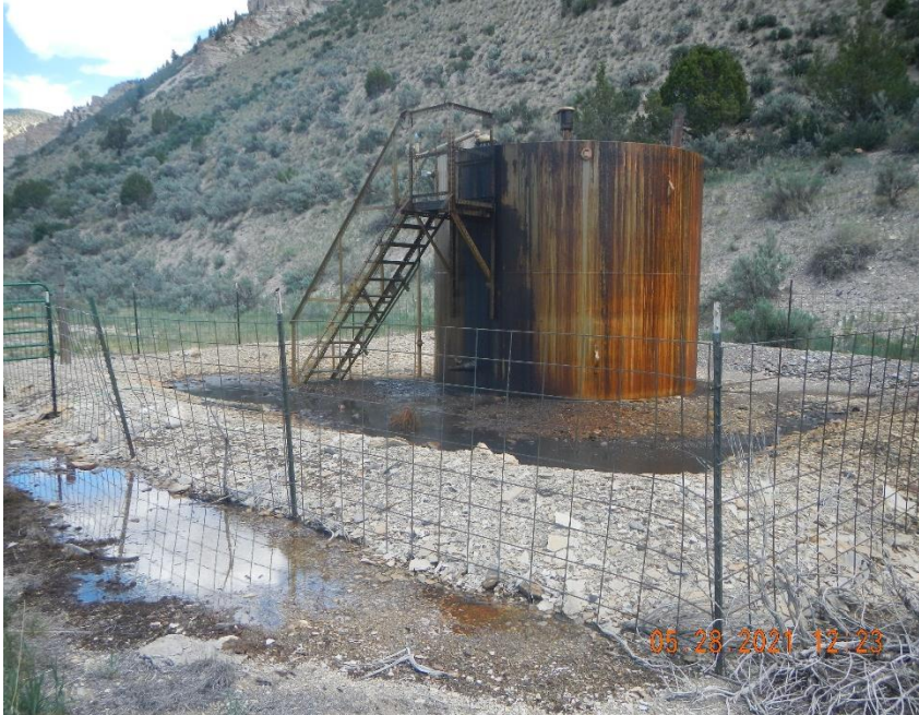
Tank overflowing and spilling into berm.
