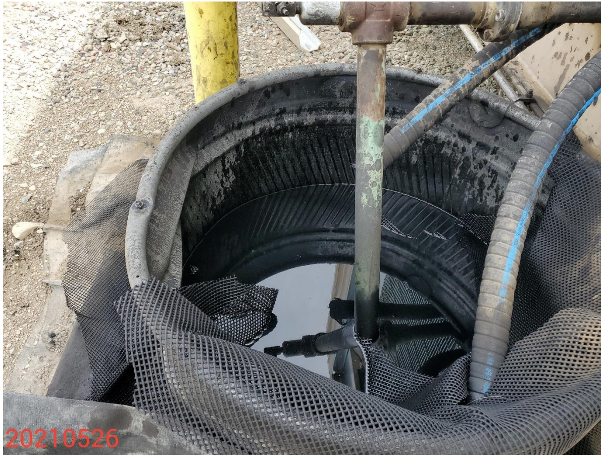
Photo 14: See comments under photo 13. Photo shows chemicals within tank. Equipment to prevent entry by wildlife missing.
