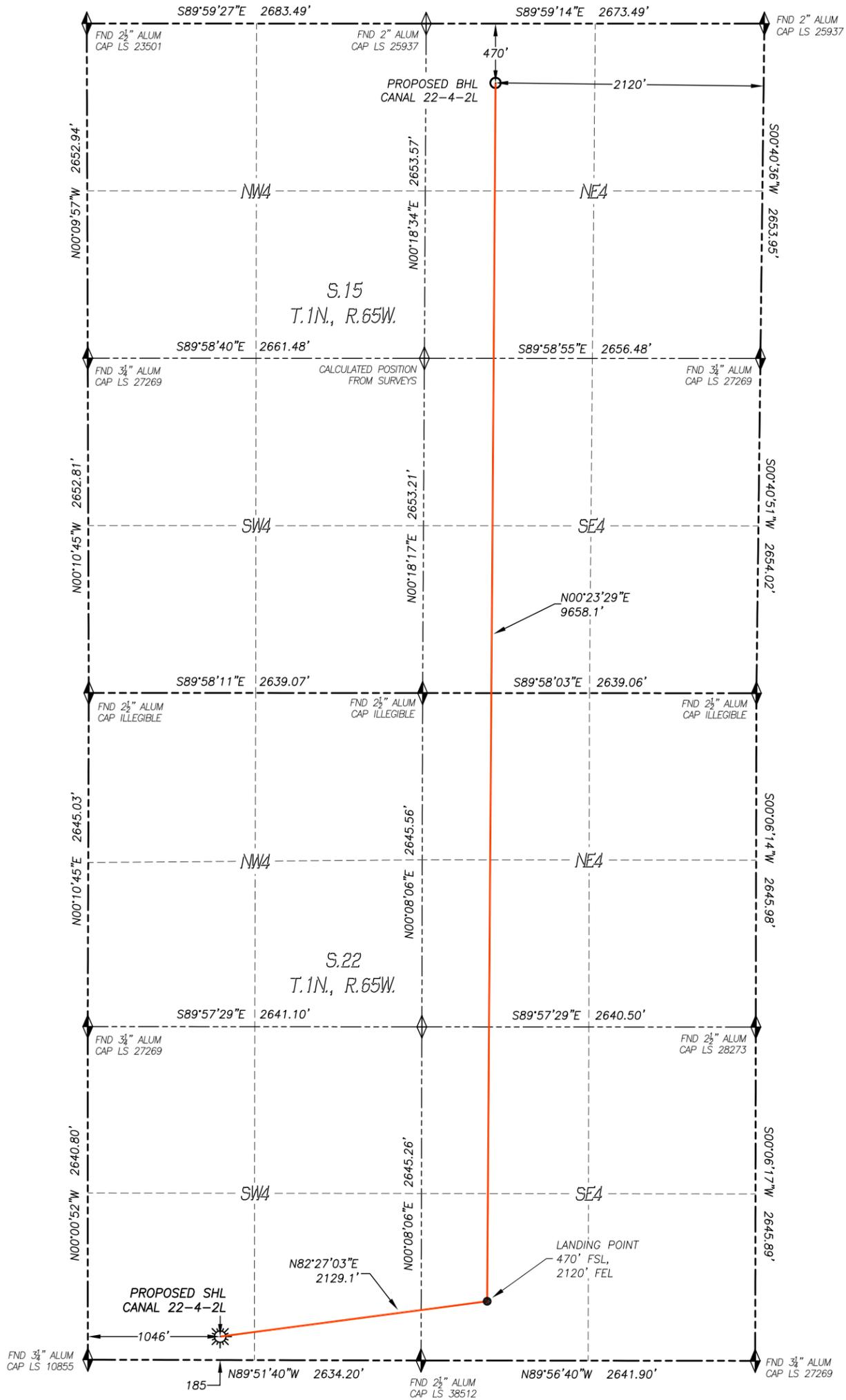
IN ACCORDANCE WITH A REQUEST FROM CONFLUENCE RESOURCES, DALEY LAND SURVEYING, INC. HAS DETERMINED THE SURFACE LOCATION OF THE CANAL 22-4-2L WELL TO BE 185' FSL, 1046' FWL, AS MEASURED AT NINETY (90) DEGREES FROM THE SECTION LINES OF SECTION 22, TOWNSHIP 1 NORTH, RANGE 65 WEST, AND THE BOTTOM HOLE LOCATION TO BE 470' FNL, 2120' FEL, AS MEASURED AT NINETY (90) DEGREES FROM THE SECTION LINES OF SECTION 15, TOWNSHIP 1 NORTH, RANGE 65 WEST, OF THE 6TH PRINCIPAL MERIDIAN, WELD COUNTY, COLORADO.
