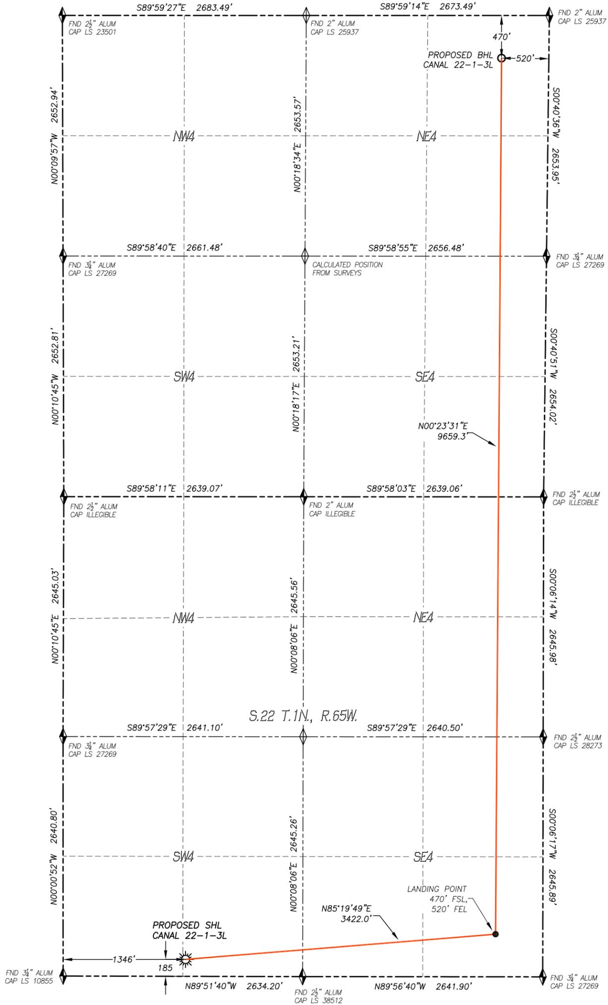
IN ACCORDANCE WITH A REQUEST FROM CONFLUENCE RESOURCES, DALEY LAND SURVEYING, INC. HAS DETERMINED THE SURFACE LOCATION OF THE CANAL 22-1-3L WELL TO BE 185' FSL, 1346' FWL, AS MEASURED AT NINETY (90) DEGREES FROM THE SECTION LINES OF SECTION 22, TOWNSHIP 1 NORTH, RANGE 65 WEST, AND THE BOTTOM HOLE LOCATION TO BE 470' FNL, 520' FEL, AS MEASURED AT NINETY (90) DEGREES FROM THE SECTION LINES OF SECTION 15, TOWNSHIP 1 NORTH, RANGE 65 WEST, OF THE 6TH PRINCIPAL MERIDIAN, WELD COUNTY, COLORADO.
