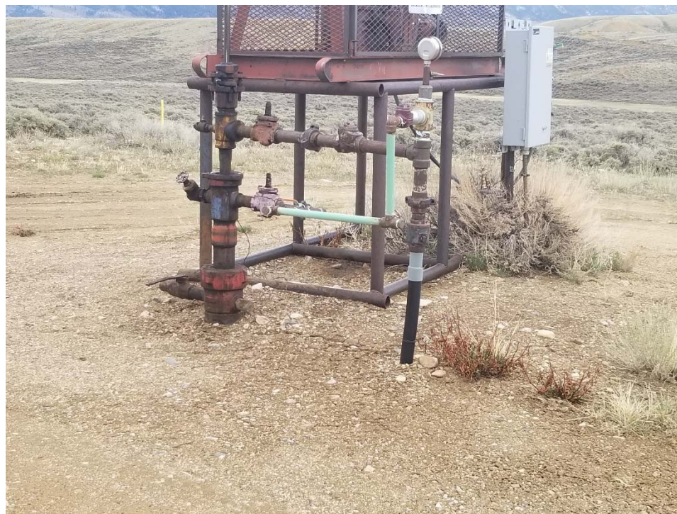
Photo 1. No bradenhead access apparent.
