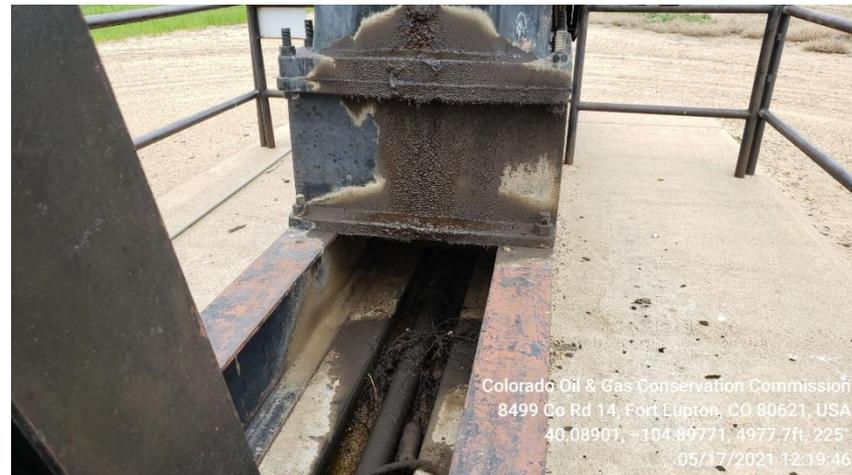
**Photo 5 Leaking plug on pump jack gear box**
