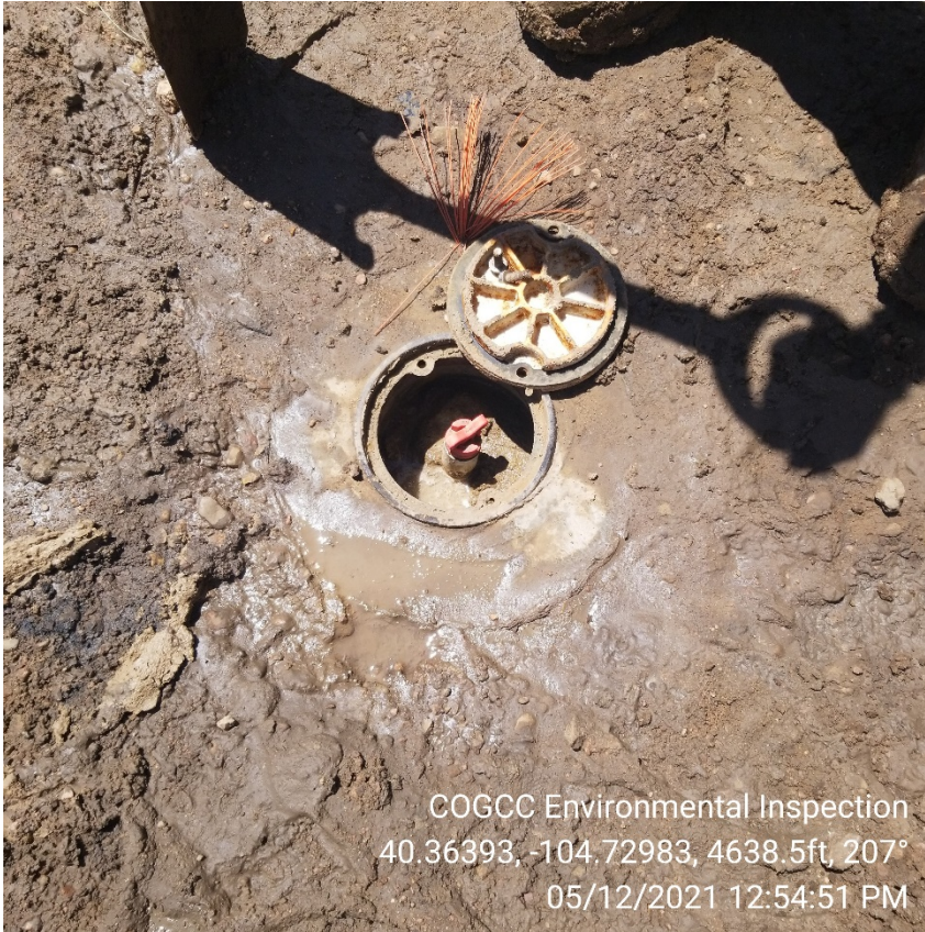
Photo 7 – The monitoring well network for Remediation Project #12644 was in the path of the flow. As of inspection all wells were visually inspected and were not impacted. Water will be sampled from these wells as part of spill cleanup.
