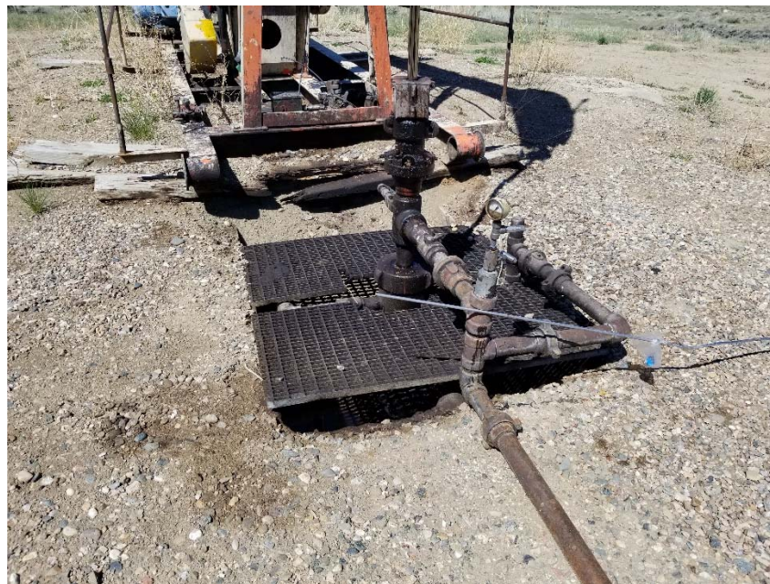
Photo 2. No bradenhead access apparent.
