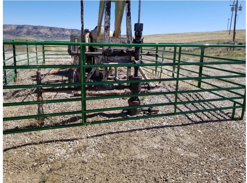
Photo 2. No bradenhead access apparent.
