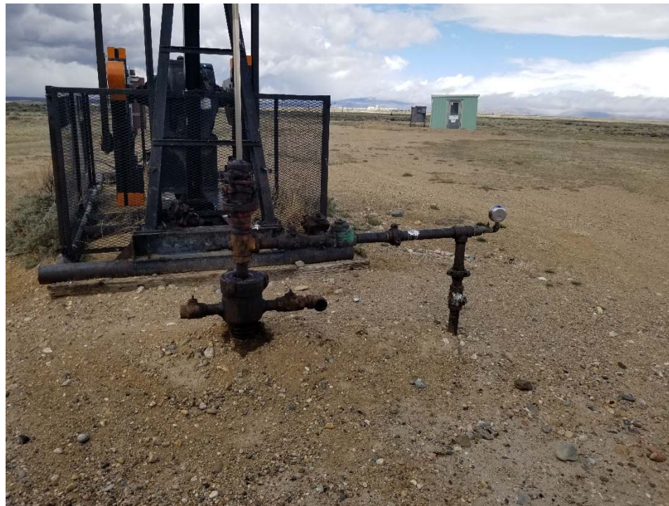
Photo 1. No bradenhead access apparent.
