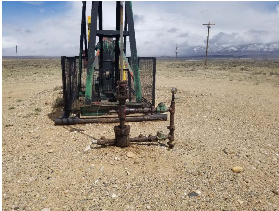
Photo 1. No bradenhead access apparent.
