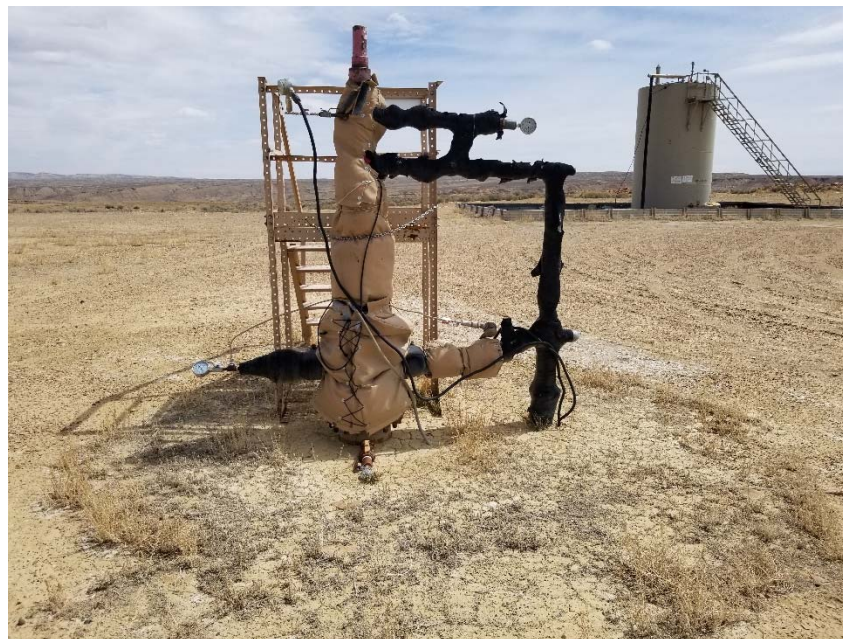
Photo 2. No bradenhead access apparent.
