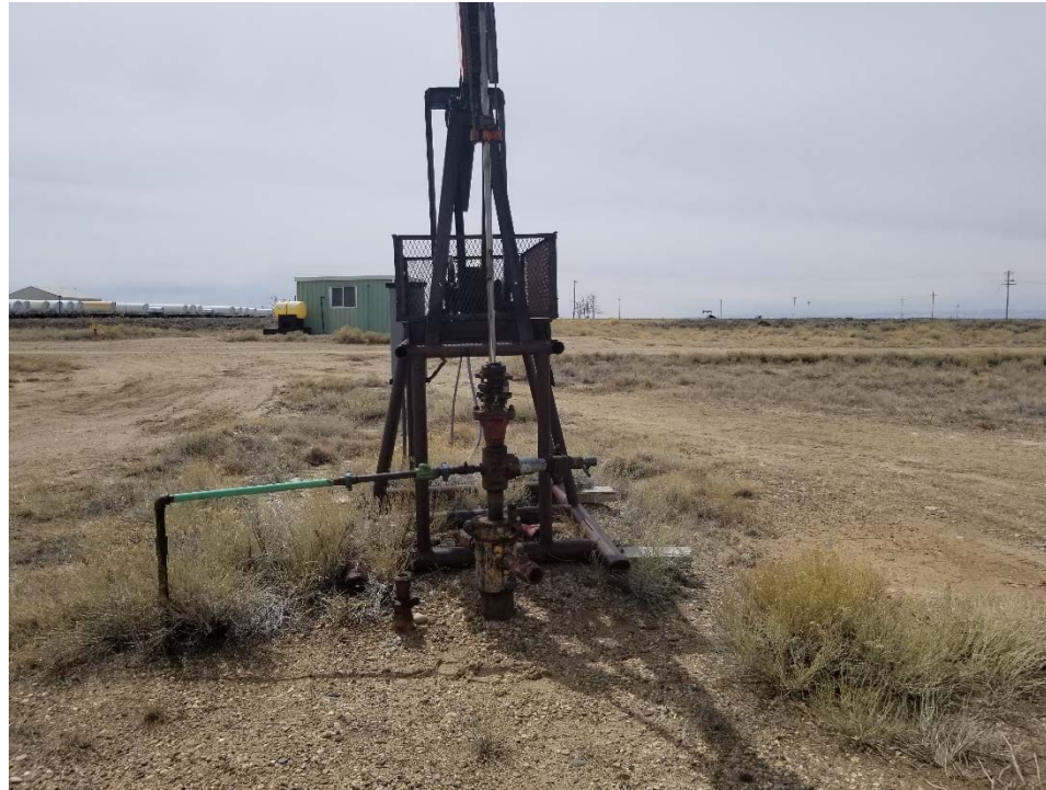
Photo 1. Overview of location taken facing southwest. No bradenhead access apparent.
