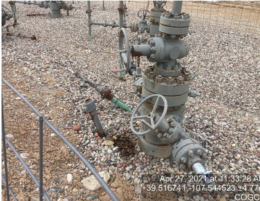
Staining under master valve
