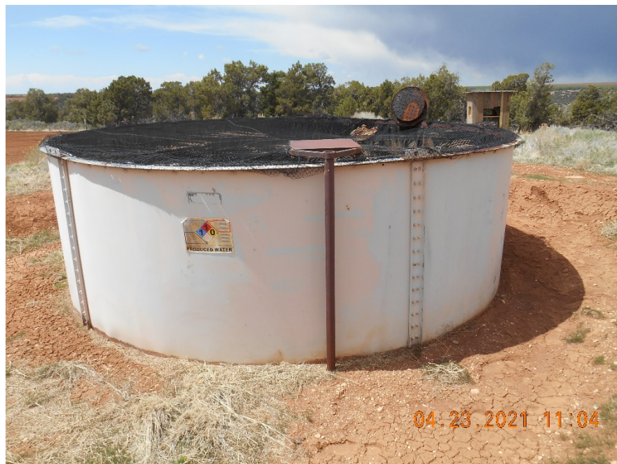
100 bbl produced water tank ½+ full of oil/water.
