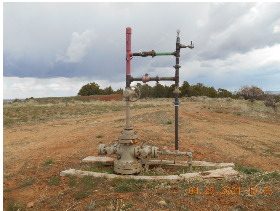
Wellhead with plunger lift.
