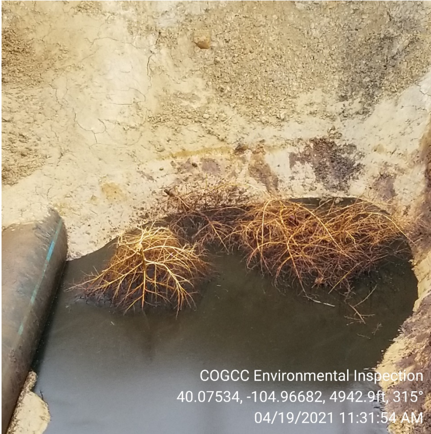
Photo 3 – Free product observed on groundwater. Flowlines exposed.
