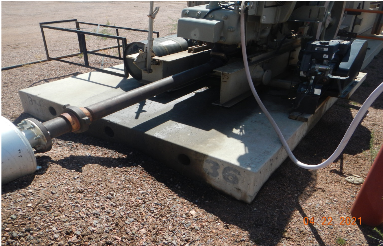
Photo 8. There is oil leaking from the pumpjack engine. Stained soil have not been cleaned up.
