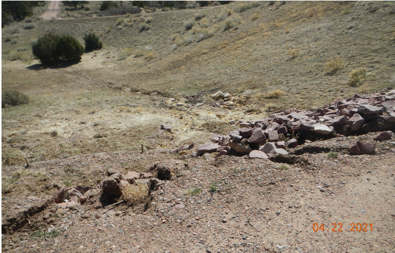
Photo 11. There is erosion occurring across the road at the north side of the location caused by stormwater directed from the top perimeter ditch shown in the previous photo. Previous corrective action has not been performed.
