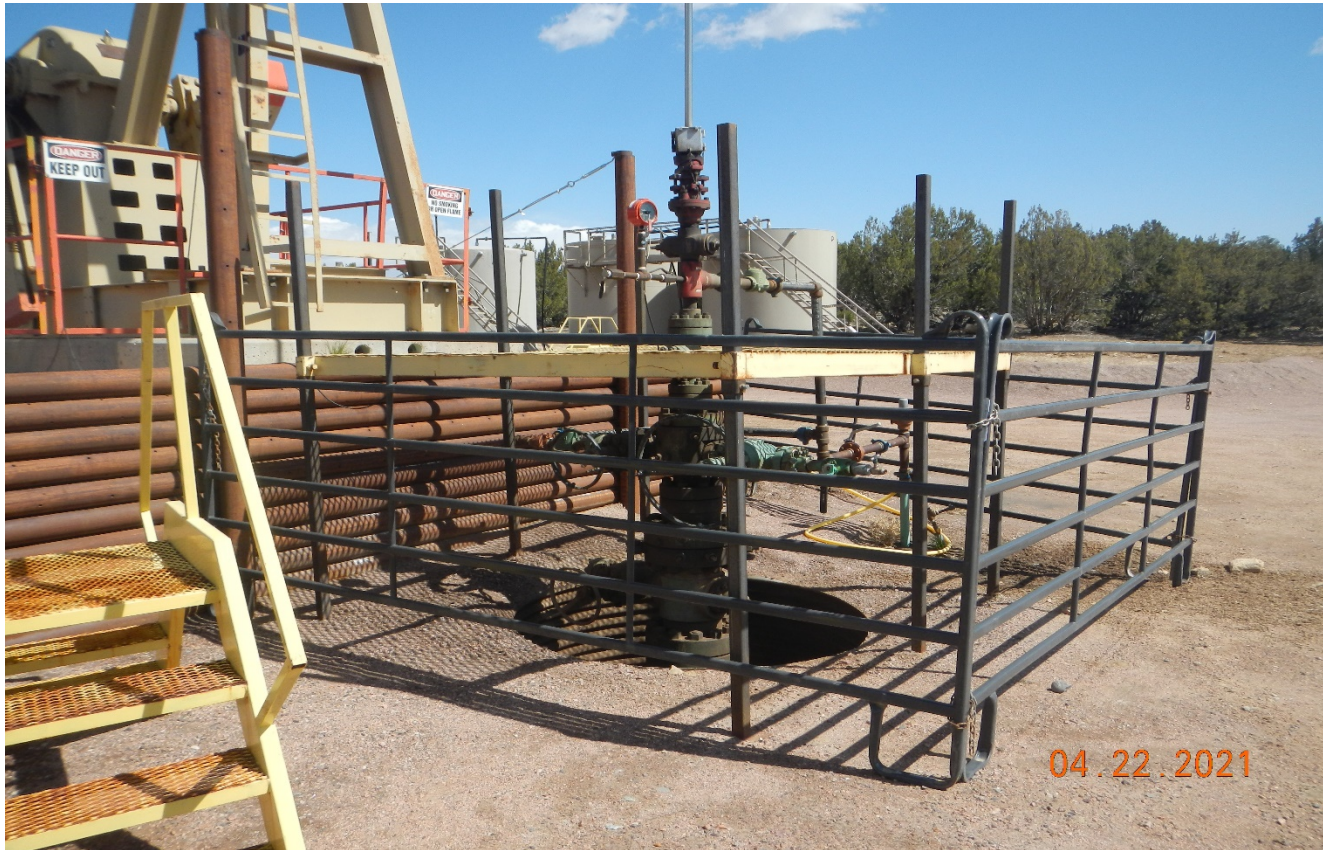
Photo 7. There was an audible gas leak heard from the wellhead. Operator was contacted during inspection of this issue.
