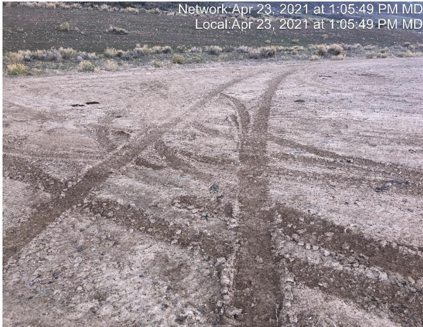
Photo #3603 location lacks stabilization
