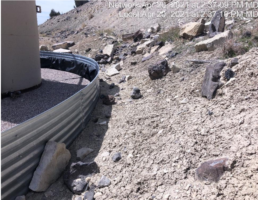
Photo #3569 Run on to location is not being effectively controlled.
