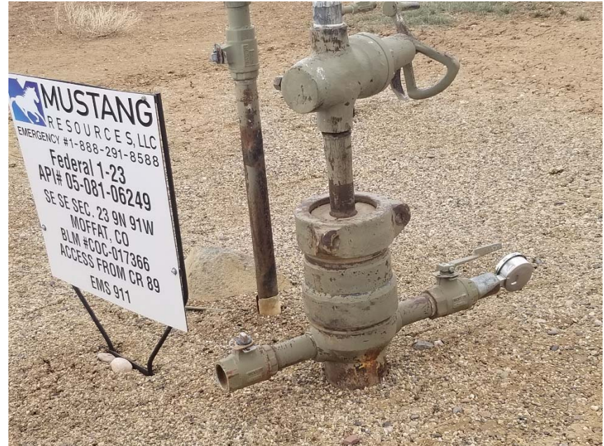
Photo 4. Wellhead sign incomplete/inaccurate. No bradenhead access apparent.
