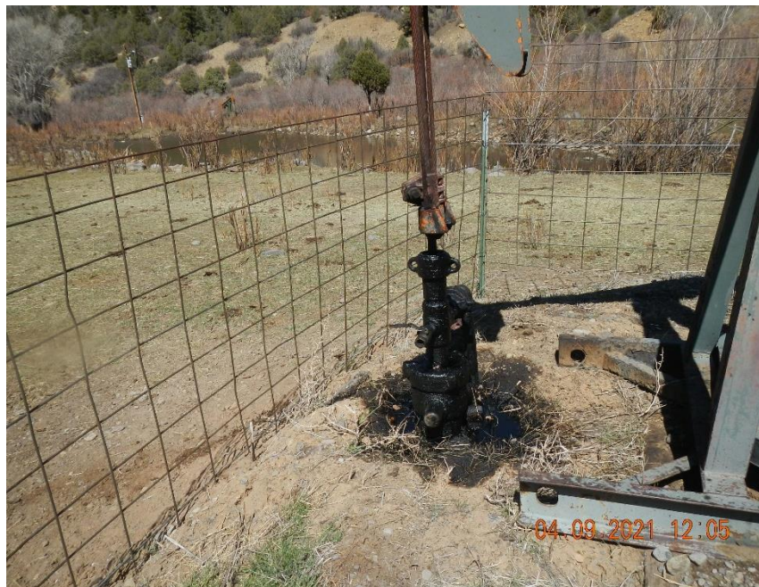
Nielson #5 well head with impacted soil and free product.
