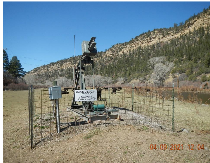
Nielson #5 well sign and pump jack. Well sign is not compliant with Rule 605.d.
