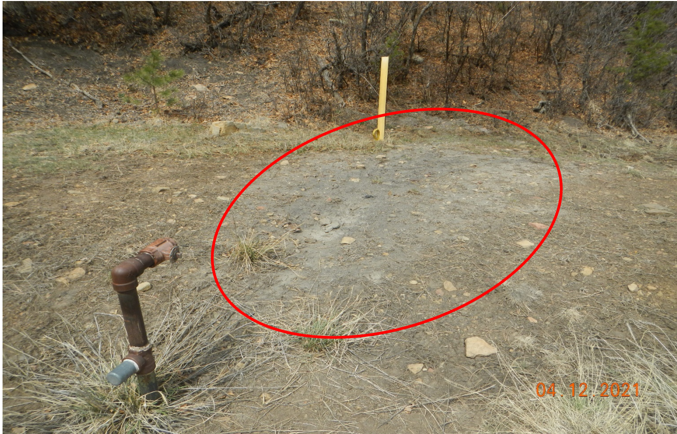
Photo 3. There is signs of produced water discharge from this pipe. There is a grey/brown in area circled.
