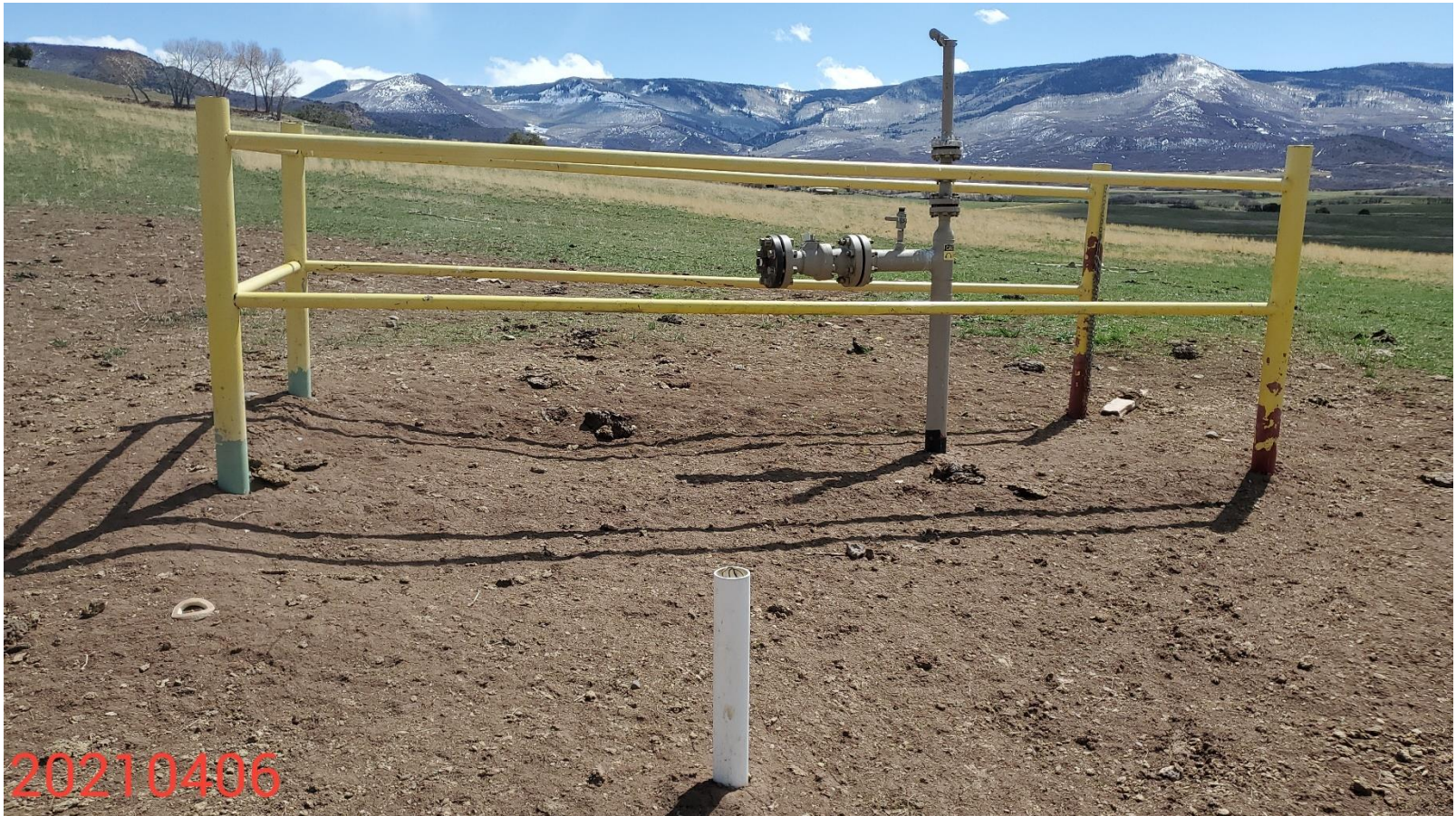
Photo 6: Photo shows surface equipment remaining on the Location; equipment requires removal pursuant with Rule 1004.a
